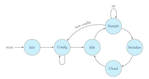
Figure 5: State diagram of module operation
