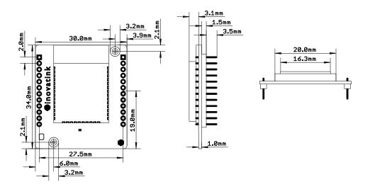
Figure 3: WIB Module's Dimensions
